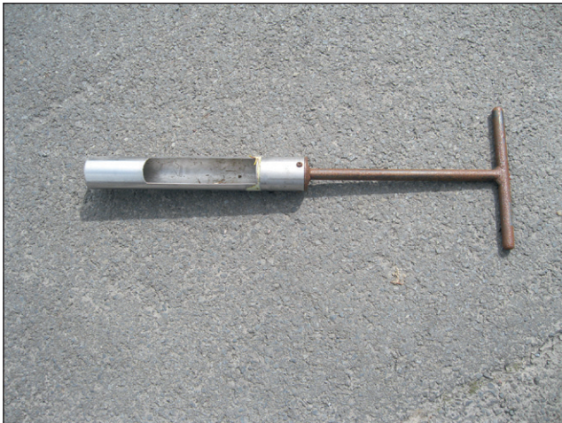
Figure 23.1 Hay bale corer. Caution is required when sampling some very high DM bales that the friction does not present a fire risk.
